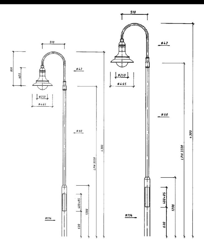
Luminaire: TML 360 Pole: TZM 701.35 Jib: TMA 412 TML 360 K TBM 7414.40
